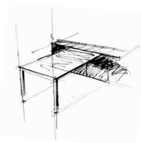
EN LA IMAGEN SE MUESTRA CÓMO LAS TAPAS SE APOYAN SOBRE PÓRTICOS Y/O SOBRE ARMARIOS INFERIORES, CREANDO UN ESPACIO MÁS DIÁFANO Y LIGERO PARA EL PUESTO DE TRABAJO • L'IMAGE MONTRÉ COMMENT LES PLATEAUX DE TABLE S'APPUIENT SUR DES PORTIQUES ET/OU SUR DES ARMOIRES INFÉRIEURES, EN CRÉANT UN ESPACE PLUS OUVERT ET PLUS LÉGER POUR LE POSTE DE TRAVAIL • THE PHOTO SHOWS HOW THE TOPS REST ON THE LEGS AND/OR LOWER CABINETS, CREATING A BRIGHTER AND LIGHTER LOOK TO THE WORK-STATION.
